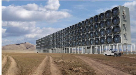
Rendering of CE's air contactor design. Source: Carbon Engineering
